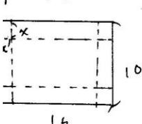
$$\begin{aligned} \text{Volume } V &= (16-x)(10-x)x = (16-2x)(10x-x^2) = 4x^3 - 32x^2 + 20x^2 + 160x \\ &= 4x^3 - 52x^2 + 160x = 4(x^3 - 13x^2 + 40x). \end{aligned}$$
