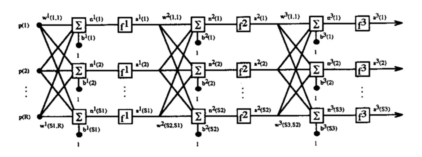
Fig. 1. Three-layer feedforward network.
