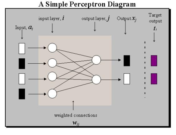
The outputs are summed across all the inputs (a[i]) received by a node (j) in the output layer. The output of each node is determined as such:
